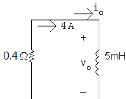
$$i_o = 4e^{-80t} \text{ A}, \quad t \geq 0$$
