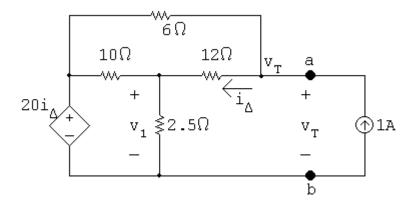
$$\frac{v_1 - 20i_{\Delta}}{10} + \frac{v_1}{2.5} + \frac{v_1 - v_T}{12} = 0$$
