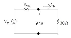
$$v_{\rm oc} = V_{\rm Th} = 75 \text{ V}; \quad i_{\rm L} = 60/30 = 2 \text{ A};$$
