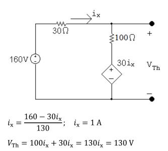
Using the test-source method to find the Thévenin resistance gives
