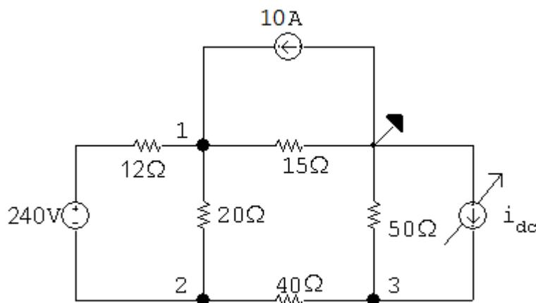
Since the 10 A source is developing 0 W,  $v_1$  must be 0 V.
