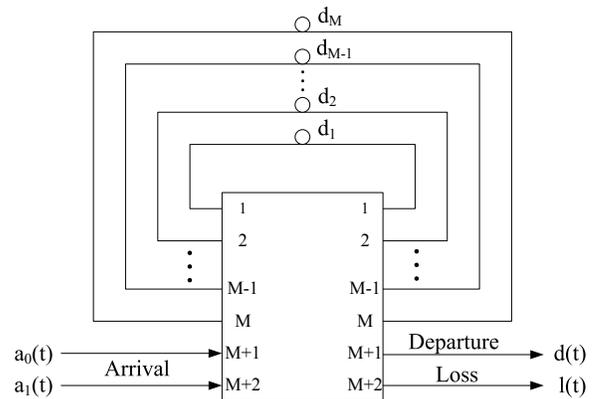
Fig. 1. A 2-to-1 FIFO multiplexer with buffer  $\sum_{i=1}^M d_i$ .
