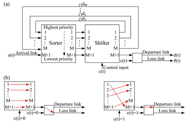
Fig. 1. (a) A construction of an optical priority queue with buffer  $\sum_{i=1}^M d_i$  (note that the sorter and the shifter can be combined together so that they can be implemented by using a single optical crossbar switch). (b) The two possible connection patterns of the shifter and the  $1 \times 2$  switch in (a).
