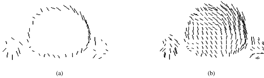
Fig. 15. (a) The displacement vectors on the three contours. (b) The interpolated displacement vectors inside the contours.
