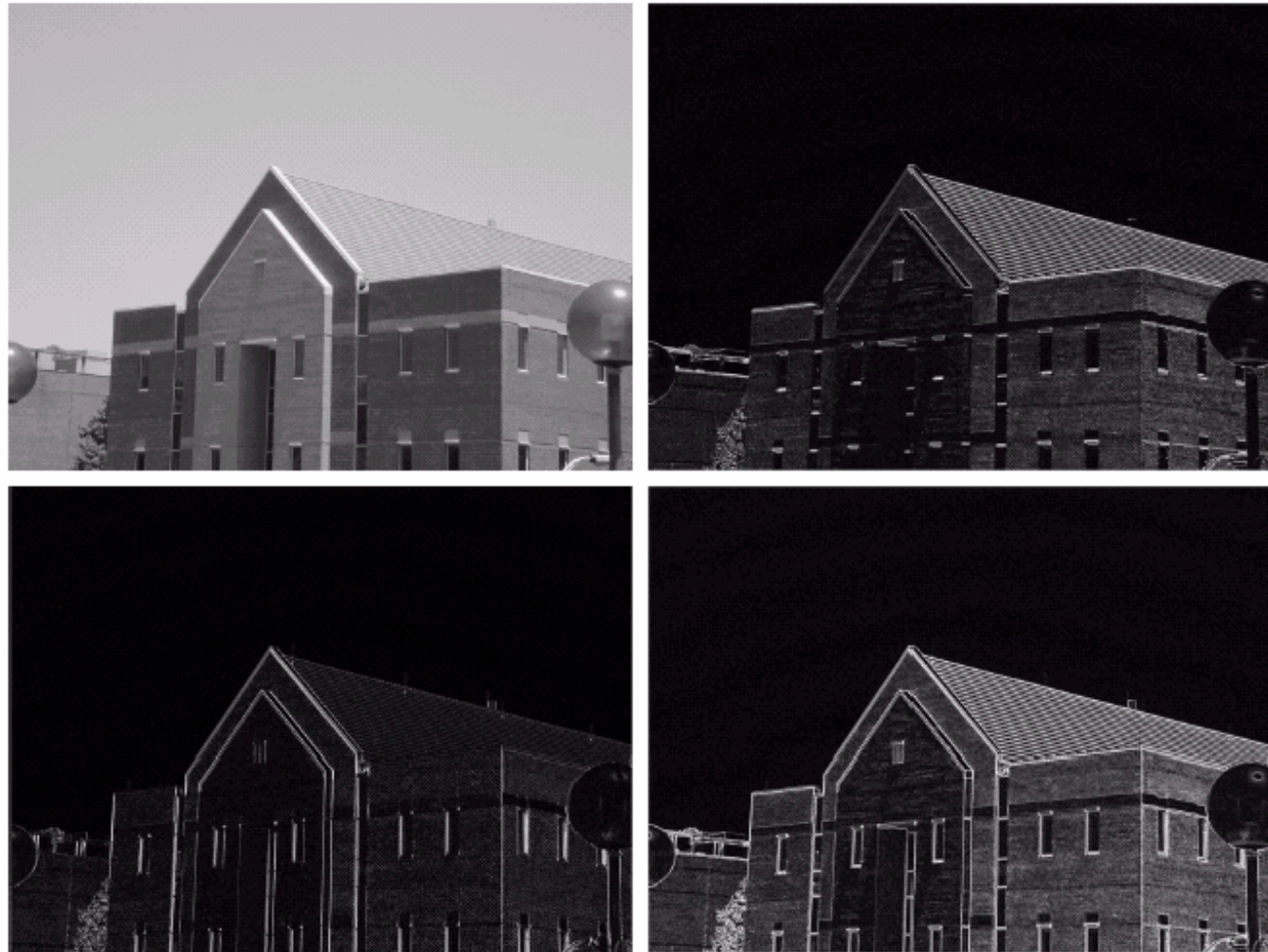
FIGURE 10.10 (a) Original image. (b) |G_x| , component of the gradient in the x -direction. (c) |G_y| , component in the y -direction. (d) Gradient image, |G_x| + |G_y| .
