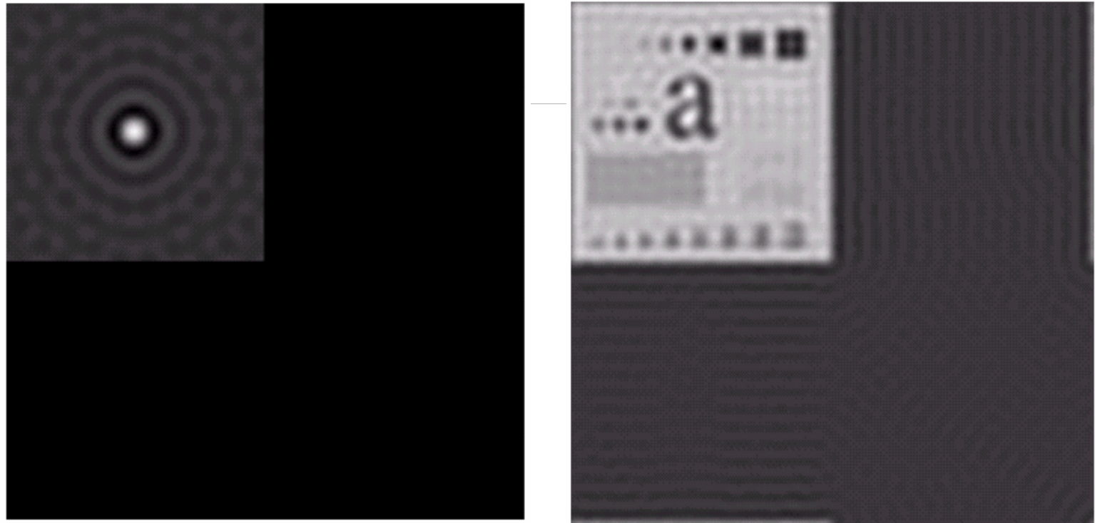
FIGURE 4.39 Padded lowpass filter is the spatial domain (only the real part is shown).
