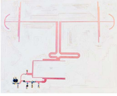
Fig. 20. Fabricated duplexing rectenna.
