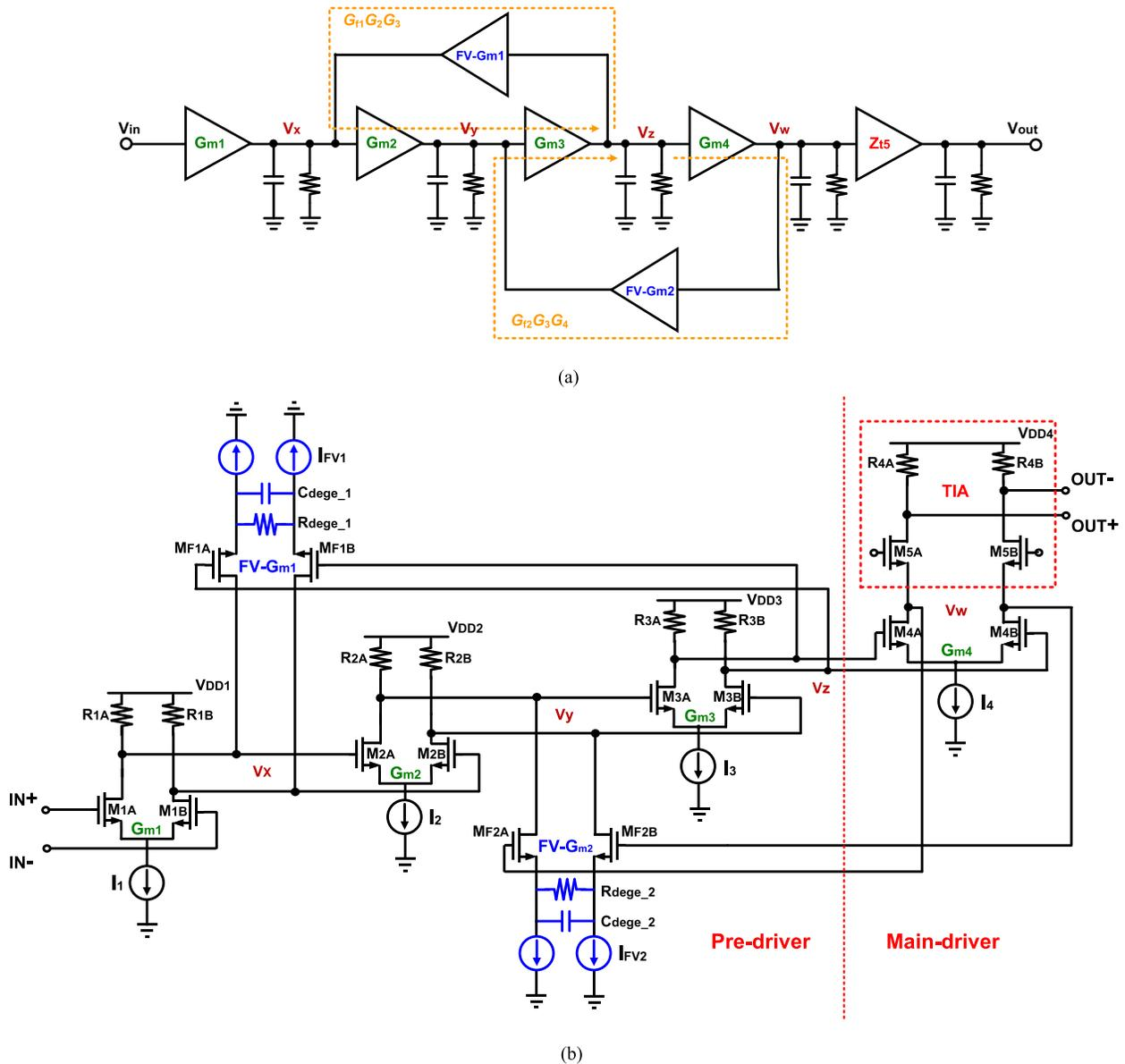
Fig. 3. (a) Block diagram of the proposed modulator driver. (b) Transistor level circuit schematic of the proposed modulator driver.
