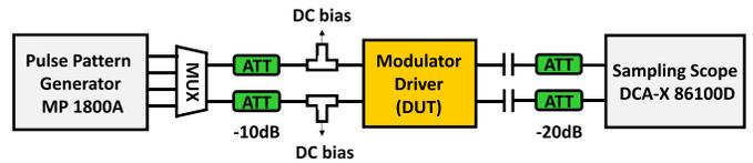
Fig. 18. PAM4 measurement setup for the modulator driver.
