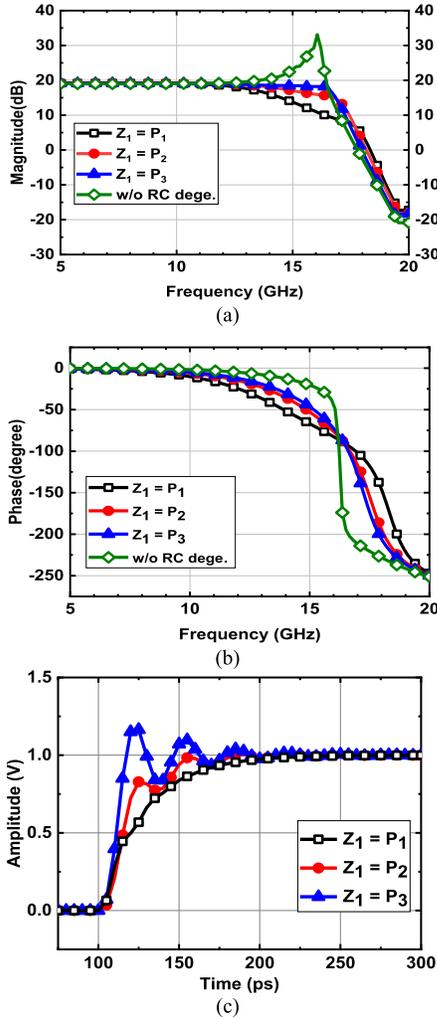
Fig. 7. Calculated Bode plots of the modulator drivers based on the simplified transfer function. (a) Magnitude. (b) Phase. (c) Time domain step response with different locations of  $z_1$ .
