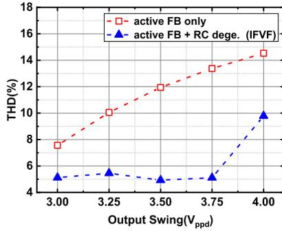
Fig. 9. Simulated THD with a 1-GHz 500 mV<sub>ppd</sub> sinusoidal input signal as a function of the output swing. The increased output level is achieved by reducing the feedback factor of the active feedback loop using the current sources.
