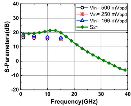
Fig. 15. Comparison of the simulated frequency response of the IFVF modulator driver under different input swing levels with  $S_{21}$ .
