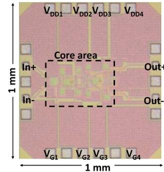
Fig. 16. Micrograph of the proposed IFVF modulator driver in 90-nm CMOS.
