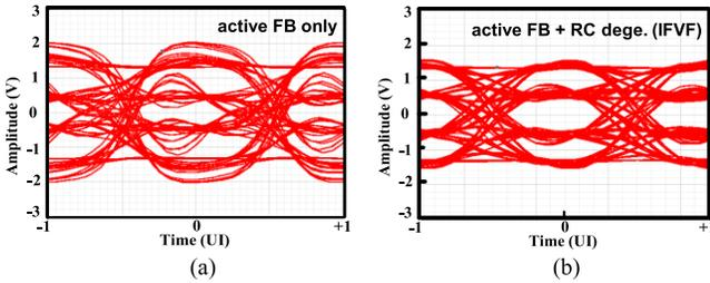
Fig. 13. Simulated result of 20 Gbauds PAM-4 signals. (a) Active feedback only and (b) active feedback w/i RC degeneration in the active feedback loops.
