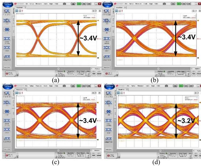
Fig. 19. Measured results of NRZ eye diagram. (a) 10, (b) 20, (c) 25, and (d) 32 Gb/s.
