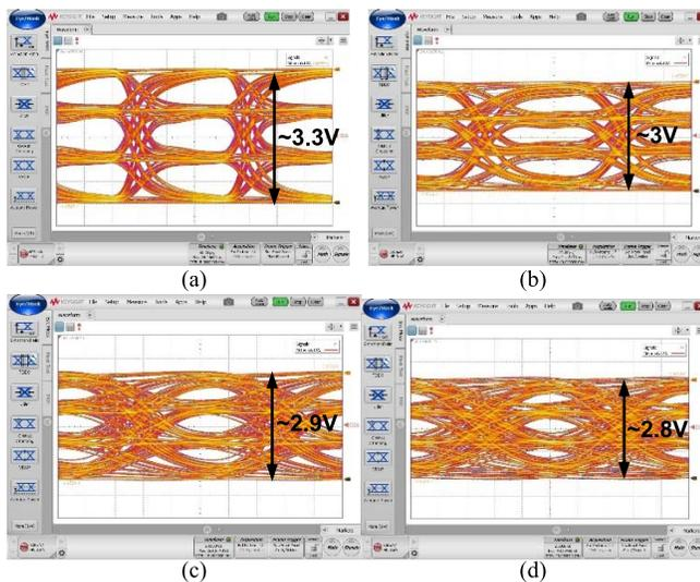
Fig. 20. Measured result of PAM4 eye diagram. (a) 5, (b) 10, (c) 15, and (d) 20 Gbaud.
