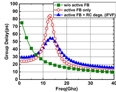
Fig. 11. Comparison of the simulated group delay of the proposed modulator driver.
