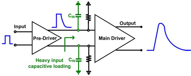
Fig. 2. Illustration of the ISI issue due to a long tail in a conventional modulator driver due to heavy capacitive loading in the main driver.
