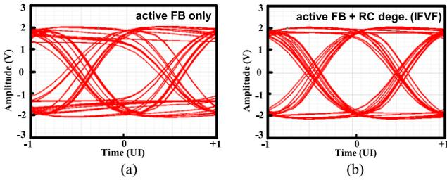
Fig. 12. Simulated 40 Gb/s NRZ eye diagrams. (a) Active feedback only and (b) active feedback w/i RC degeneration in the active feedback loops.
