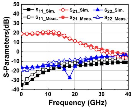
Fig. 17. Simulated and measured results of differential S-parameters of the proposed inductorless modulator driver.
