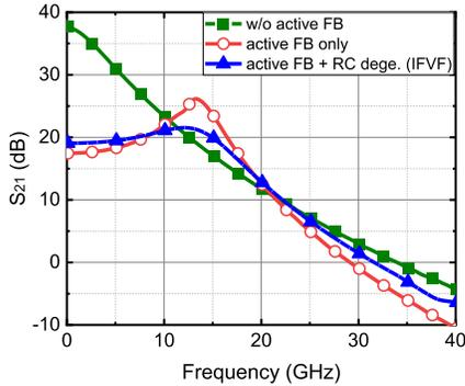
Fig. 5. Comparison of the simulated frequency responses of the modulator driver in different design cases.
