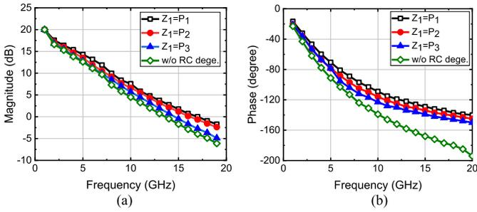
Fig. 6. Calculated Bode plots of the loop gain based on the simplified transfer function. (a) Magnitude. (b) Phase.
