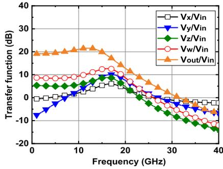
Fig. 4. Transfer functions at different nodes in the proposed modulator driver.
