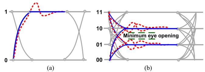
Fig. 1. Conceptual plot of the impact of signal overshoot on (a) NRZ and (b) PAM4 eye diagrams.
