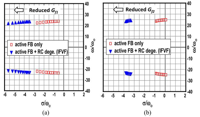
Fig. 8. Comparison of simulated pole-zero plots of the modulator driver w/i and w/o IFVF by sweeping the voltage gain of the two active feedback cells. (a)  $G_{f1}$  and (b)  $G_{f2}$ , respectively.
