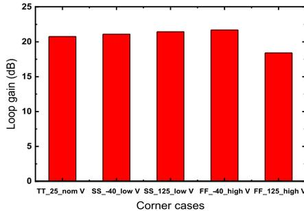
Fig. 14. Simulated loop gain of the proposed IFVF modulator driver in different corner cases.
