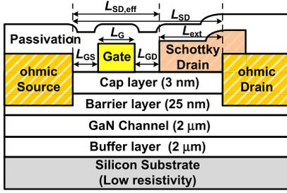
Fig. 1. Cross section of the AlGaIn/GaN HEMT on silicon substrate.
