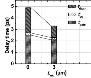
Fig. 12. Comparison of each delay component of the HEMTs with/without Schottky extension.
