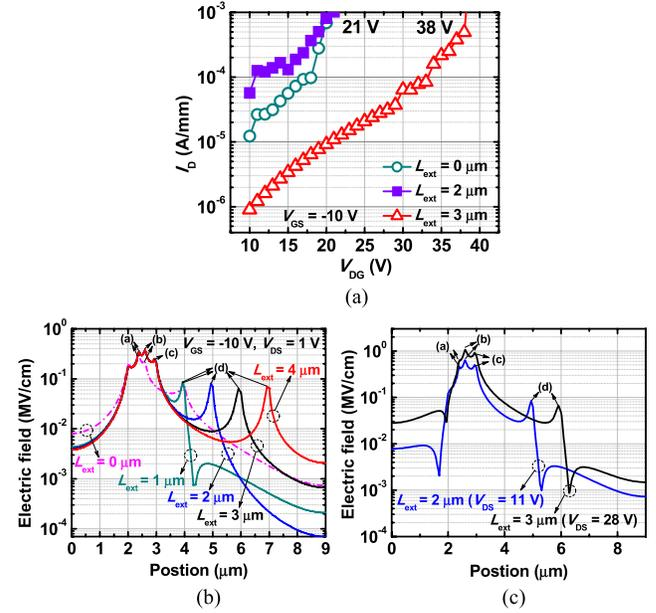
Fig. 5. (a) Measured three-terminal OFF-state breakdown characteristics. (b) Simulated  $E$ -field distribution for  $V_{GS} = -10 \text{ V}$  and  $V_{DS} = 1 \text{ V}$  with different values of  $L_{ext}$ . (c) Simulated  $E$ -field distribution of the devices for  $L_{ext} = 2$  and  $3 \mu\text{m}$  with the bias conditions corresponding to Fig. 5(a) when breakdown occurs.
