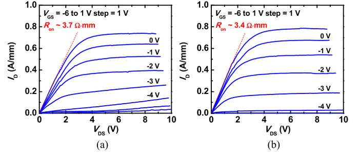
Fig. 2.  $I_D$ – $V_{DS}$  characteristics of the GaN-on-Si HEMTs ( $W_G = 2 \times 50 \mu\text{m}$ ) for (a)  $L_{ext} = 0 \mu\text{m}$  and (b)  $L_{ext} = 3 \mu\text{m}$ .
