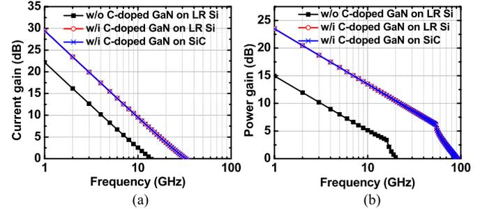
Fig. 13. Comparison of simulated (a) Power gain and (b) Current gain for GaN HEMTs on different substrates with/without the C-doped buffer layer.
