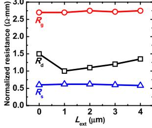
Fig. 7. Extracted parasitic resistances of the GaN-on-Si HEMTs with various  $L_{\text{ext}}$  based on the small-signal model.
