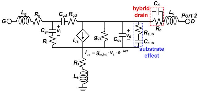
Fig. 6. Modified small-signal equivalent circuit model for the GaN-on-Si HEMTs with hybrid drain and substrate effect.
