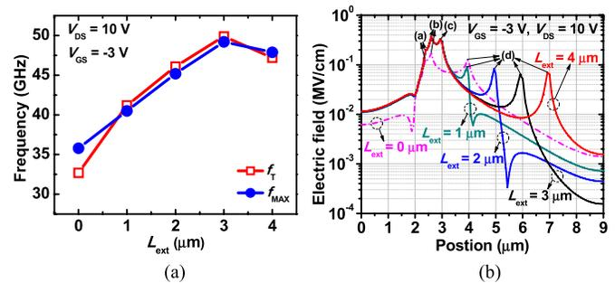
Fig. 10. (a) Measured  $f_T$  and  $f_{\text{MAX}}$  for the GaN-on-Si HEMTs ( $W_G = 2 \times 50 \mu\text{m}$ ). (b) Simulated  $E$ -field distribution for  $V_{\text{GS}} = -3 \text{ V}$  and  $V_{\text{DS}} = 10 \text{ V}$  with different values of  $L_{\text{ext}}$ .
