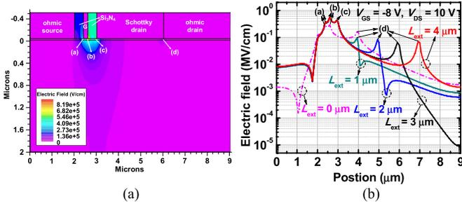
Fig. 4. TCAD simulation of the hybrid drain devices. (a) Device structure for  $L_{ext} = 3 \mu\text{m}$ . (b)  $E$ -field distribution for  $V_{GS} = -8 \text{ V}$  and  $V_{DS} = 10 \text{ V}$ .
