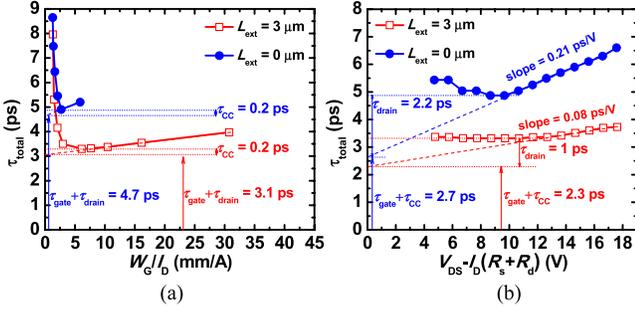
Fig. 11. Total delay time  $\tau_{\text{total}}$  as a function of (a) Inverse drain current density and (b) Voltage across the channel under the gate.
