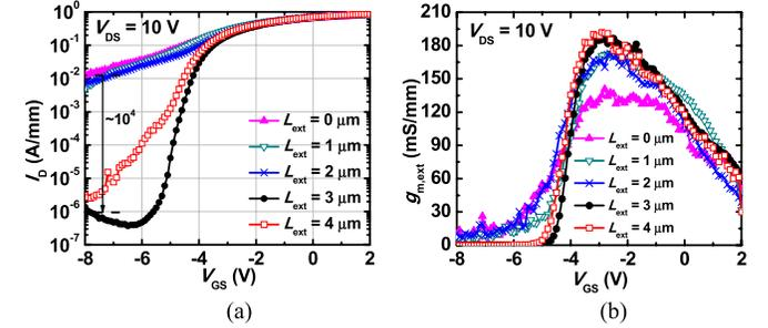
Fig. 3. Measured dc characteristics for (a)  $I_D$ – $V_{GS}$  and (b)  $g_{m,ext}$ – $V_{GS}$  at  $V_{DS} = 10 \text{ V}$ .
