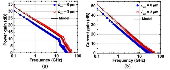
Fig. 9. GaN-on-Si HEMTs with/without Schottky extension for (a) power gain and (b) current gain comparison ( $V_{\text{GS}} = -3$  V and  $V_{\text{DS}} = 10$  V).
