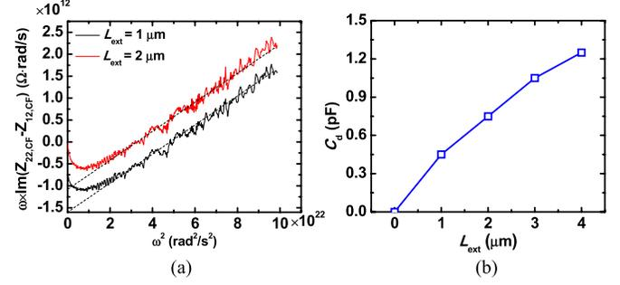
Fig. 8. (a) Parameter extraction procedure of  $C_d$  for  $L_{\text{ext}} = 1$  and 2  $\mu\text{m}$ . (b) Extracted  $C_d$  as a function of  $L_{\text{ext}}$ .
