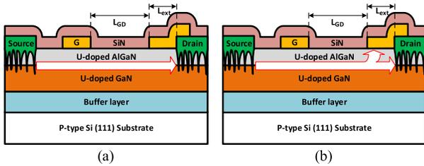
Fig. 1. ON-state current mechanism of AlGaIn/GaN HEMTs with hybrid Schottky-ohmic drain. (a) When Schottky drain diode is OFF ( $V_{DS} < V_{ON,SK}$ ), the current flows only via ohmic conduction. (b) When Schottky drain diode is ON ( $V_{DS} > V_{ON,SK}$ ), the current via Schottky electrode rapidly increases.
