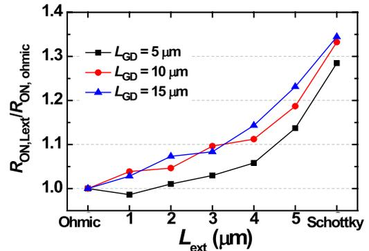
Fig. 3. Normalized  $R_{ON}$  as a function of  $L_{ext}$  for  $L_{GD}$  of 5, 10, and  $15 \mu\text{m}$ .
