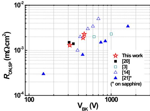
Fig. 7. Comparison of the FoM ( $V_{BK}^2/R_{ON,sp}$ ) for the proposed hybrid drain devices ( $L_{ext} = 2 \mu\text{m}$  and  $L_{GD} = 5, 10, \text{ and } 15 \mu\text{m}$ ) with other GaN-based devices in the previous publications.
