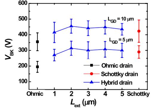
Fig. 5. Measured OFF-state breakdown voltage  $V_{\text{BK}}$  ( $V_{\text{GS}} = -10 \text{ V}$ ) as a function of the extended Schottky drain length  $L_{\text{ext}}$ .
