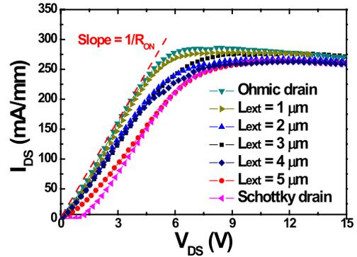
Fig. 2. Comparison of  $I_{DS}-V_{DS}$  characteristics for three types of devices with  $L_{GD} = 5 \mu\text{m}$  at  $V_{GS} = 1 \text{ V}$ .
