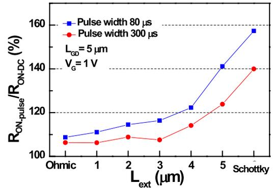
Fig. 8. Normalized  $R_{ON}$  versus  $L_{ext}$  in pulsewidths of 80 and 300  $\mu\text{s}$ .
