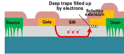
Fig. 9. Location of surface traps in hybrid drain devices responsible for the observed current collapse when the device is in OFF-state.
