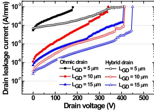
Fig. 4. OFF-state drain leakage current with  $L_{\text{ext}} = 2 \mu\text{m}$  ( $V_{\text{GS}} = -5 \text{ V}$ ).
