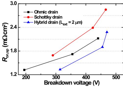
Fig. 6. Measured  $V_{BK}$  versus  $R_{ON,sp}$  of the Schottky drain, ohmic drain, and hybrid drain devices with  $L_{ext} = 2 \mu\text{m}$  and  $L_{GD} = 5, 10, \text{ and } 15 \mu\text{m}$  for comparison.
