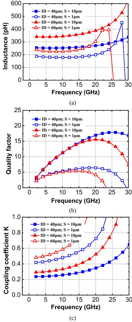
Fig. 5. Simulated results of the proposed fully 3-D symmetrical TSV (1:1) transformers with different geometries, including (a) inductance, (b)  $Q$  factor, and (c) coupling coefficient  $K$ .
