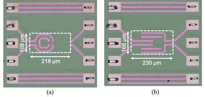
Fig. 8. Chip photograph of (a) fully 3-D symmetrical TSV 1:1 transformer with an inner diameter of  $40\ \mu\text{m}$ . (b) Differential symmetrical TSV 1:3 transformer.
