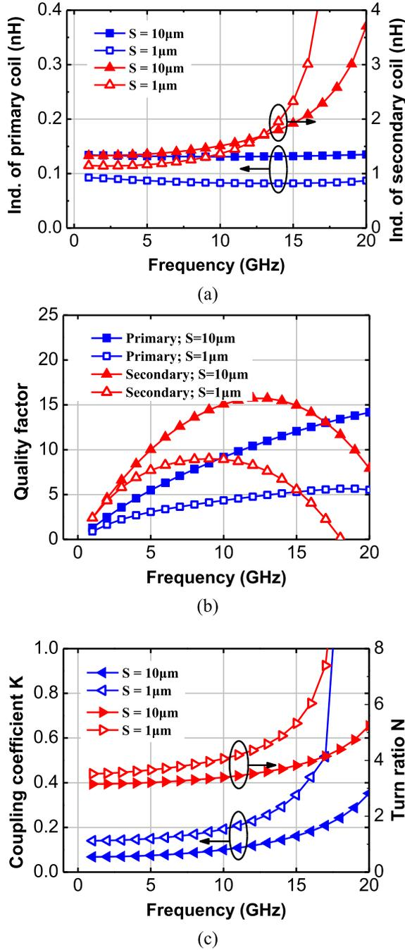
Fig. 7. Simulated results of the proposed differential symmetrical TSV monolithic (1:3) transformer. (a) Inductance. (b)  $Q$  factor. (c) Coupling coefficient  $K$  and turn ratio with various geometries.
