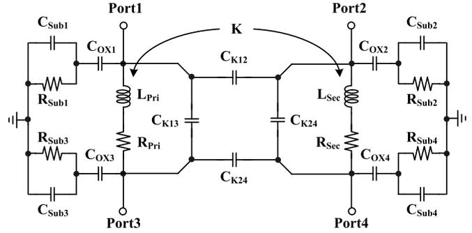
Fig. 9. Equivalent-circuit model of 3-D symmetrical TSV 1:1 transformer.
