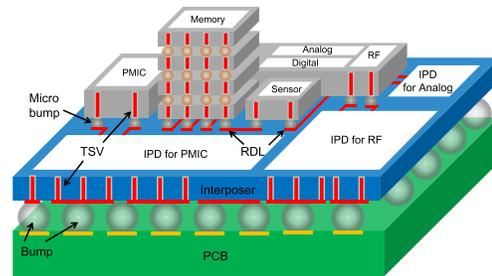
Fig. 1. Conceptual plot of heterogeneous 3-D IC integration with an interposer IPD.
