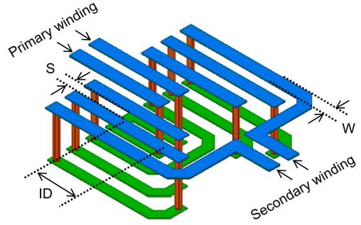
Fig. 6. Proposed 3-D TSV 1: $N$  transformer, where the primary winding is one and that for the secondary coil is 3.
