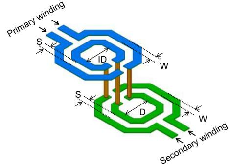
Fig. 4. Primary and secondary windings of the proposed 3-D fully symmetric TSV monolithic (1:1) transformer.
