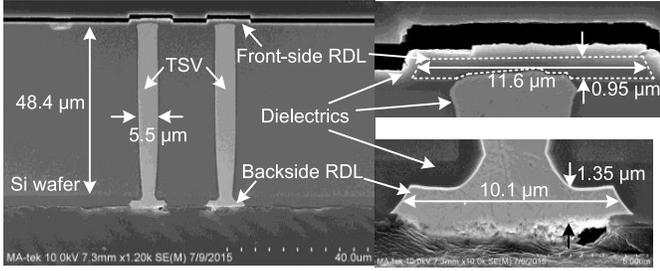
Fig. 3. Cross-sectional SEM image of the TSV region of the 3-D transformer.
