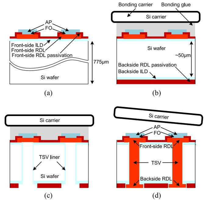
Fig. 2. Process flow of the in-house developed 3-D IC via-last backside-TSV interposer. (a) Front-side process. (b) Wafer thinning and backside layer deposition. (c) TSV etching. (d) Carrier removing.
