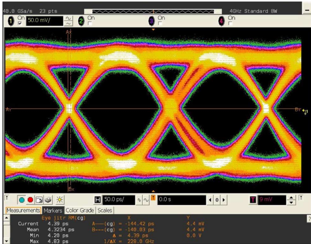
Fig. 15. Measured eye-diagram of Chip-1 (4-to-1 MUX-FF) at 6 Gbits/s.
