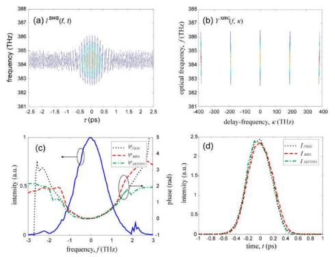
Fig. 3. (a) Experimentally measured interferometric spectrogram, and (b) its Fourier transform with respect to delay. For clarity, Fig. 3b is manipulated to highlight the components around  $\kappa = \pm f_0$ . (c) Spectral phase profiles, and (d) temporal intensity profiles measured by FROG (dotted), MIFA (dashed), and MEFISTO (dash-dot), respectively. The solid line in Fig. 3c represents the fundamental power spectrum measured by OSA.
