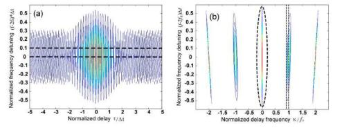
Fig. 1. (a) Simulated interferometric spectrogram of a transform-limited Gaussian pulse defined in the main text, and (b) its Fourier transform with respect to delay. (For clarity, Fig. 1b is manipulated to highlight the components around  $\kappa = \pm f_0$ )
