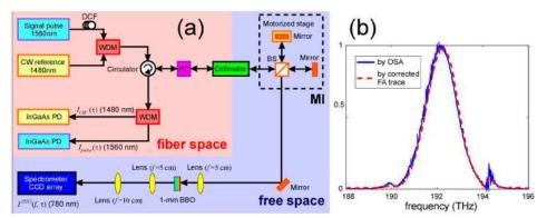
Fig. 2. (a) Experimental setup of interferometric spectrogram measurement. DCF: dispersion compensating fiber. WDM: wavelength division multiplexer. PC: polarization controller. BS: beam splitter. MI: Michelson interferometer. PD: Photodetector. (b) Fundamental power spectra of the signal pulse measured by an optical spectrum analyzer (OSA) (solid), and fringe-corrected field autocorrelation (FA) trace (dashed), respectively.
