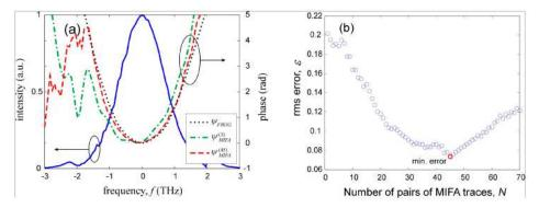
Fig. 5. (a) Spectral phase profiles measured by MIFA using 1 (dash-dot), and 45 (solid) pairs of MIFA traces sampled from the interferometric spectrogram, respectively. The spectral phase measured by FROG at SNR = 28 (dotted) is shown as a reference. (b) rms error value versus the number of pairs of MIFA traces used for retrieving the spectral profile by Eq. (3).
