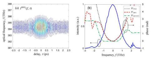
Fig. 4. (a) Experimentally measured interferometric spectrogram of the signal pulse broadened by a 1.9-m-long SMF. (b) Spectral phase profiles measured by FROG (dotted), MIFA (dashed), and MEFISTO (dash-dot), respectively. The solid line represents the fundamental power spectrum measured by OSA.
