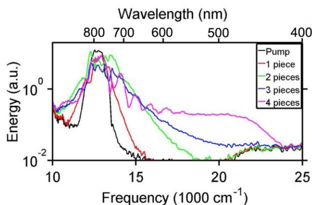
Figure 2. The broadband spectrum with different number of thin plates of crystal.
