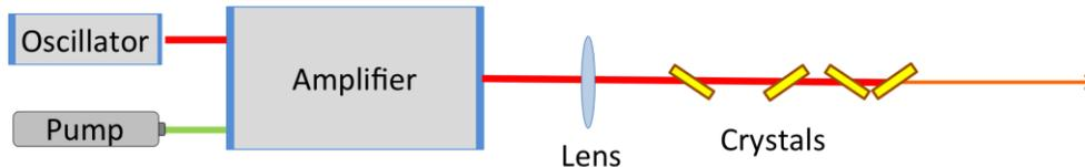
Figure 1. Schematic of the experimental setup. A supercontinuum spectrum can be generated by a single beam focused onto multiple pieces of thin fused silicas aligned consecutively down the beam path.
