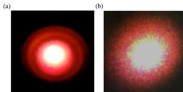
Figure 3. Image of transverse profile of generated supercontinuum beam (a) from four thin plates and (b) from a thick plate.
