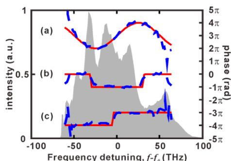
Fig. 4. Power spectrum (shaded). The three types of spectral phases added by the shaper (solid) and retrieved by MIFA (dashed), respectively.
