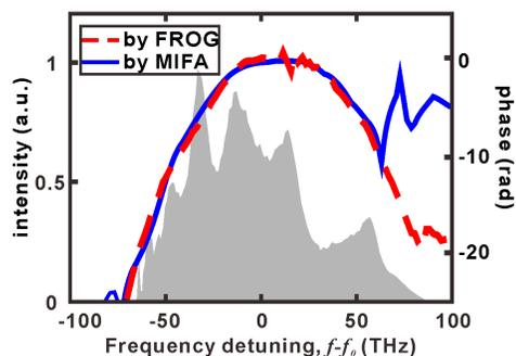
Fig. 2. Power spectrum measured by a spectrometer (shaded), and the spectral phases retrieved by FROG (dashed) and MIFA (solid), respectively.
