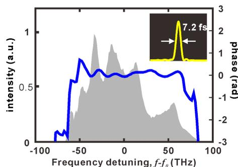
Fig. 3. Power spectrum (shaded), and the residual spectral phase retrieved by MIFA (solid). Inset: The corresponding temporal intensity.
