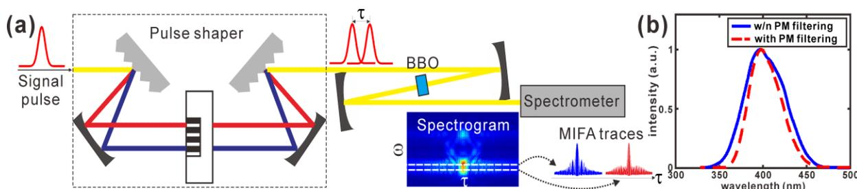
Fig. 1. (a) Experimental setup. (b) SHG power spectra of a TL pulse without (solid) and with (dashed) phase-matching (PM) filtering.
