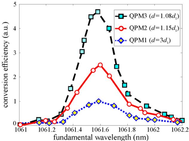
Fig. 3. (Color online) The experimentally measured phase-matching tuning curves of QPM1 (diamonds), QPM2 (circles), and QPM3 (squares), respectively.
