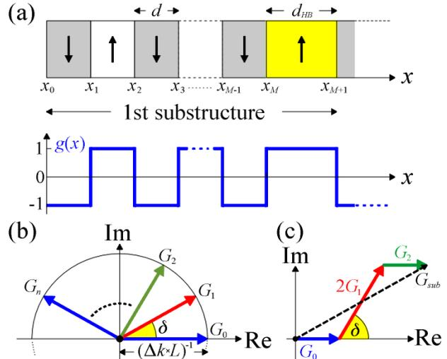
Fig. 1. (Color online) (a) Schematic of HB-QPM and the corresponding domain orientation distribution function  $g(x)$ . (b) The complex numbers  $\{G_n\}$  contributed by regular domains of length  $d=(1+\Delta)d_1$ , where  $\delta=\Delta\pi$ . (c) The complex numbers  $\{G_n\}$  and  $G_{sub}$  due to the individual domain boundaries (solid) and the entire substructure (dashed) with  $M=1$ .
