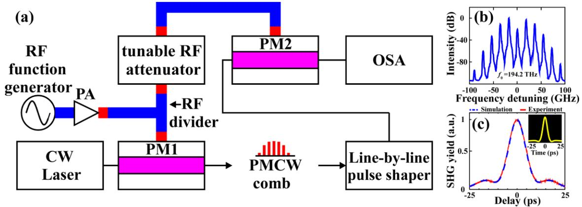
Fig. 1. (a) Experimental setup. PM: phase modulator. PA: power amplifier. (b) Power spectrum of the PMCW comb. (c) The IA functions obtained by simulation (dashed) and experiment (solid) for the corresponding TL pulse (inset).
