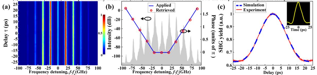
Fig. 3. Measurement of  $\psi_2(\omega)$ . (a) PROOF trace. (b) Power spectrum (shaded), applied (solid), and retrieved (circles) spectral phases, (c) Simulated (dashed) and experimentally measured (solid) IA functions. The inset shows the temporal intensity of the test pulse.
