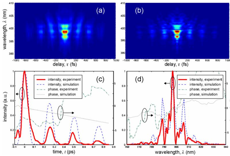
Fig. 1. (a) Measured, and (b) retrieved FROG traces when using mask M4 and a pinhole of 50  $\mu$ m in diameter. The measured and simulated intensity and phase curves in the (c) time, and (d) frequency domains, respectively.
