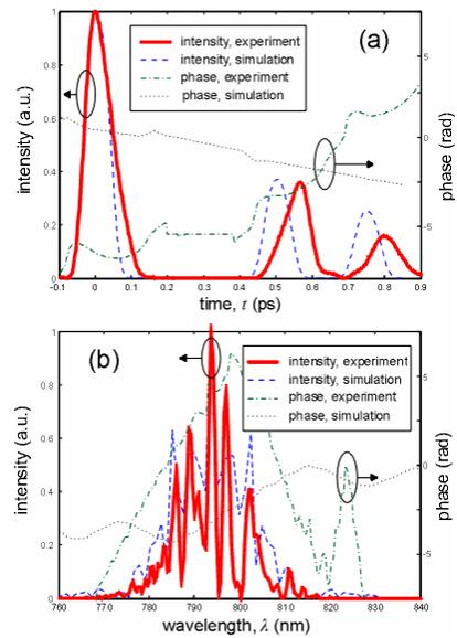
Fig. 2. The measured and simulated intensity and phase curves in the (a) time, and (b) frequency domains, respectively; when using mask M3 and a pinhole of 20  $\mu$ m in diameter.
