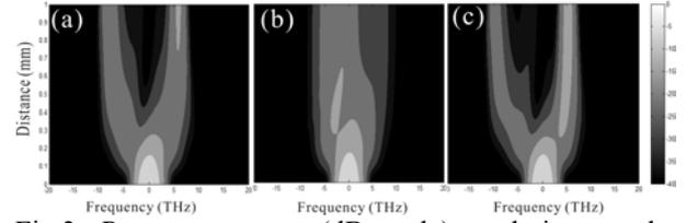
Fig.3. Power spectrum (dB scale) evolution as the Gaussian pulse propagates through waveguide with (a) ZGVD, (b) increasing normal dispersion, and (c) anomalous GVD.
