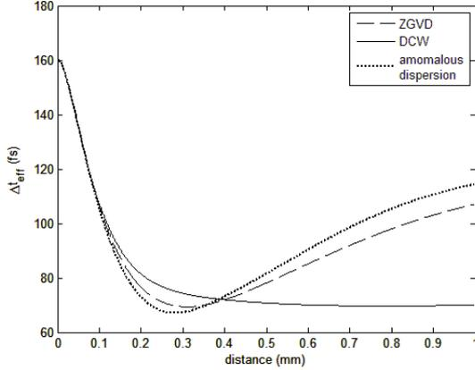
Fig.2. Effective pulse width  $\Delta t_{eff}$  versus propagation distance for ZGVD (dashed), DCW (solid), and anomalous GVD (dotted).
