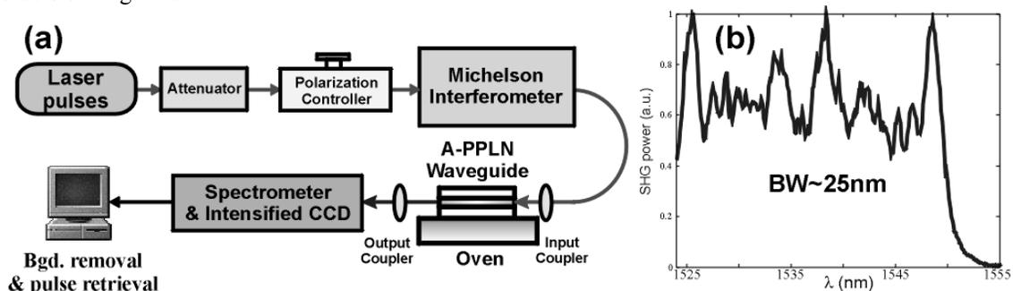
Fig. 1. (a) Experimental setup. (b) Room temperature phase-matching tuning curve of the A-PPLN waveguide.
