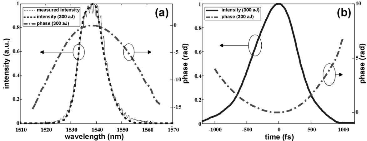
Fig. 4. Retrieved pulse depicted in: (a) frequency domain; and (b) time domain at 300-aJ coupled pulse energy. The retrieved temporal FWHM is 796 fs, and the dispersion is estimated as -70 fs/nm.
