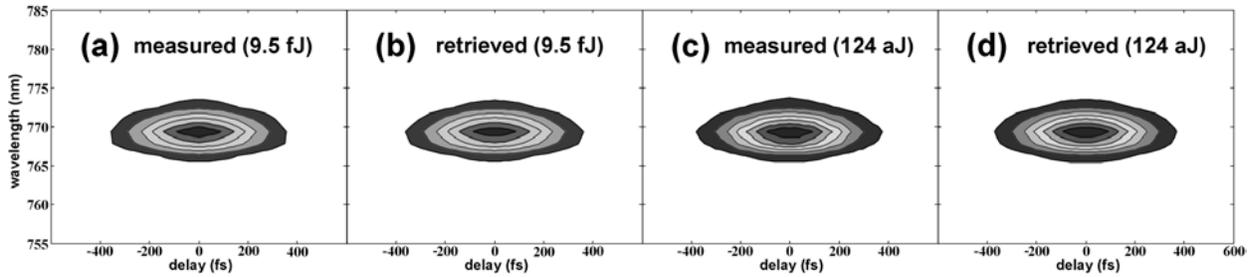
Fig. 2. FROG traces of (a) measured (b) retrieved at 9.5 fJ; and (c) measured (d) retrieved at 124 aJ.
