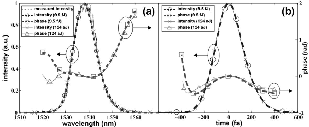
Fig. 3. Retrieved pulse depicted in: (a) frequency domain, and (b) time domain for both 9.5-fJ and 124-aJ coupled pulse energies. Dotted curve in (a) represents the independently measured power spectrum. The retrieved temporal FWHM is  $\sim 280$  fs, and the residual dispersion is about 4.2 fs/nm.
