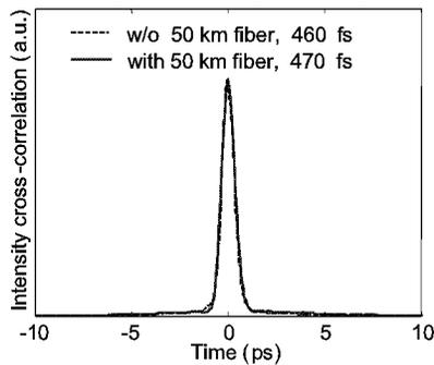
Fig. 2. Intensity cross-correlation with and without SMF/DCF module, demonstrating the distortionless 50 km fiber transmission for sub-500 fs pulse
