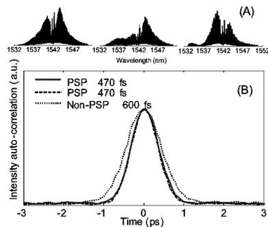
Fig. 5. (A) Spectrum variation caused by PMD. (B) Intensity auto-correlation for different polarization (PSP vs. non-PSP) at fiber link input.
