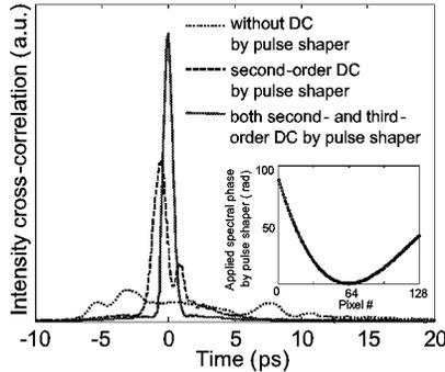
Fig. 3. Intensity cross-correlation for different pulse shaper settings. The inset figure shows the phase profile applied by pulse shaper.
