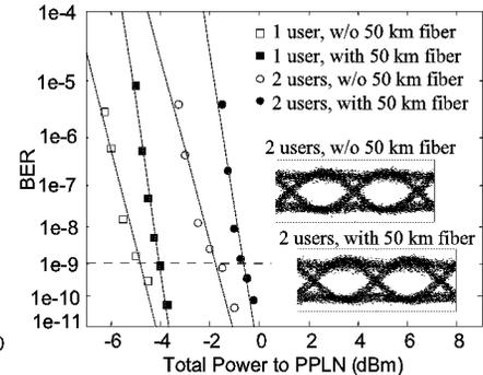
Fig. 7. BER performance for the O-CDMA system with and without 50 km fiber transmission. The inset figures show the eye diagrams for 2 users.
