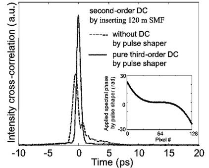
Fig. 4. Intensity cross-correlation for different pulse shaper settings by inserting 120 m SMF for complete second-order DC. The inset figure shows the phase profile applied by the pulse shaper.
