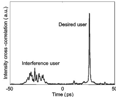
Fig. 6. Intensity cross-correlation for a 2 user O-CDMA system after 50 km fiber transmission.
