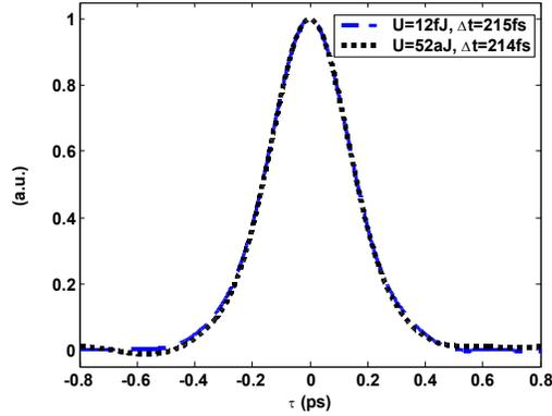
Fig. 1. Autocorrelation traces using a chirped A-PPLN waveguide (SHG BW=25 nm) with different input power levels
