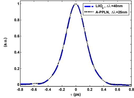
Fig. 2. Autocorrelation traces using bulk LiIO<sub>3</sub> and A-PPLN waveguide
