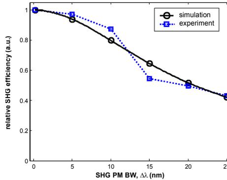
Fig. 3. Relative SHG efficiency versus SHG BW. The simulation (circle) assumes bandwidth-limited input pulses with a power spectrum same as that used in the experiment (square), and squared-shape SHG PM spectra with full widths  $\Delta\lambda$ .
