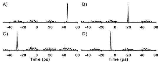
Fig. 2 Intensity cross-correlation measurements of properly decoded channels 1 to 4 (A to D respectively) demonstrating the ability to selectively decode any of the four user channels.
