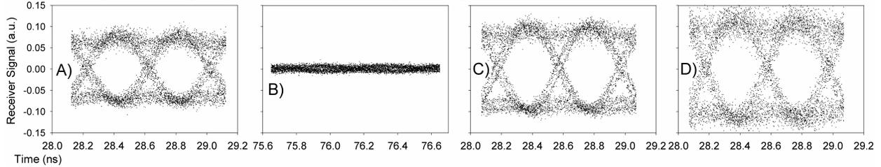
Fig. 4 Eye-diagrams after nonlinear processing (measurement point  $\beta$  in Fig. 1B), at -3dBm per user. (A) Properly decoded channel 1, single user. B) Improperly decoded channel 1, single user. C) Two user system, properly decode channel 1. D) Four user system, properly decode channel 4. A&B demonstrate the large contrast between a properly and improperly decoded single user channel. C&D demonstrate clear decoding of the desired user in a multiple user system via nonlinear processing.
