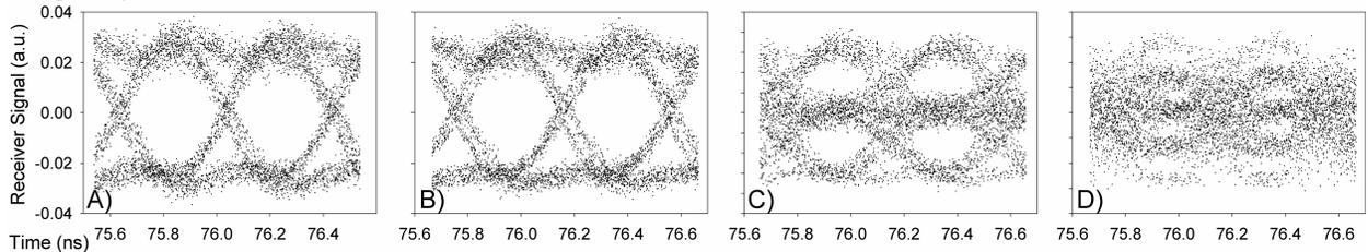
Fig. 3 Eye diagrams prior to nonlinear processing (measurement point  $\alpha$  in Fig. 1B). Single user properly decoded (A), improperly decoded (B), two user (C), and four user (D). A & B demonstrate that both properly decoded and improperly decoded single user channels look essentially identical on a linear detector. C & D demonstrate that multiple users can not be adequately separated using linear detection.
