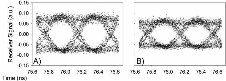
Fig. 6 Eye diagrams for properly decoded channel using alternative code families: A) quaternary code, B) Quadratic Residue code. These data demonstrate substantial flexibility in code choice.
