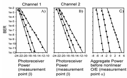
Fig. 5 Bit Error Rate measurements for single user (circles), 2 user (squares), 4 users (triangles). A) decode channel 1, B) decode channel 2, C) same as (A) but now power refers to value in nonlinear waveguide. System is operated at less than 1mW per user.
