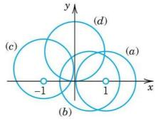
$\frac{z^2+1}{z^2-1} = \frac{z^2+1}{(z+1)(z-1)}. \text{ Circles } (a-b) \text{ only enclose } z=z_0=1, \Rightarrow f(z) = \frac{z^2+1}{z+1}, \ l=2\pi i \cdot f(1)=2\pi i.$  Circle (c) only encloses  $z=z_0=-1, \Rightarrow f(z)=\frac{z^2+1}{z-1}, \ l=2\pi i \cdot f(-1)=-2\pi i.$  Circle (d) encloses no singularity,  $\Rightarrow \frac{z^2+1}{(z+1)(z-1)}$  is analytic inside circle (d), l=0.
