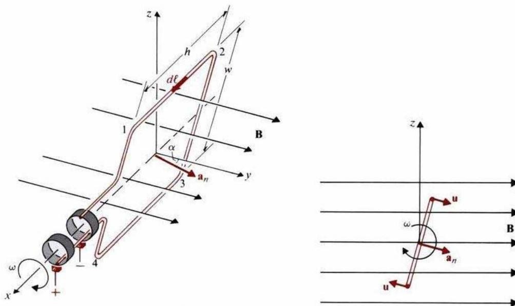
Fig. 14-6. AC generator made by a rotating a metal loop in time-varying M-field (after DKC).
