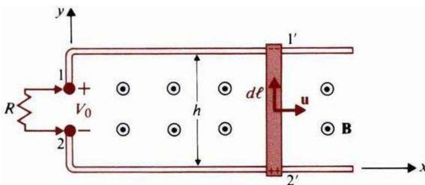
Fig. 14-4. DC generator made by a moving metal bar (after DKC).
