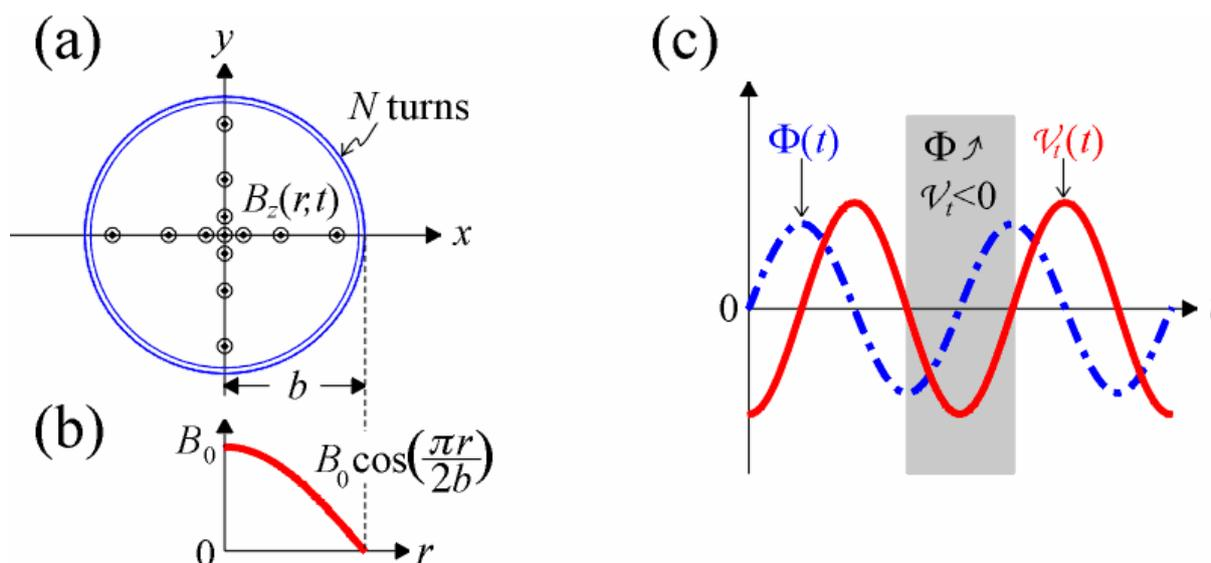
Fig. 14-1. (a) The geometry of a stationary conducting loop, and (b) the spatial amplitude of magnetic flux density passing through it. (c) The resulting magnetic flux (dash-dot) and transformer emf (solid).
