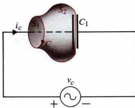
Fig. 14-7. Displacement current in a parallel-plate capacitor (after DKC).
