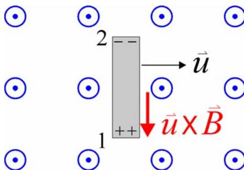
Fig. 14-3. A conductor moving in a magnetic field will induce motional emf.
