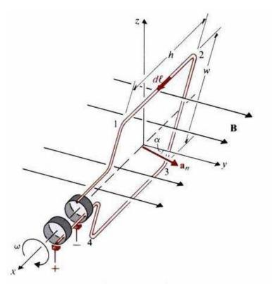
$$\Phi_{dynm} = \int_{S} \vec{B} \cdot d\vec{s} = (\vec{a}_{y} B_{0} \sin \omega t) \cdot (\vec{a}_{n} h w)$$
