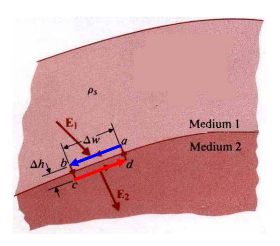
$$\oint_{C} \vec{E} \cdot d\vec{l} = \left| -\int_{S} \frac{\partial \vec{B}}{\partial t} \cdot d\vec{s} \right|$$
