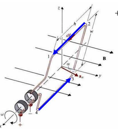
$$+ \int_{4}^{3} \left[ \left( -\vec{a}_{n} \frac{w}{2} \omega \right) \times \left( \vec{a}_{y} B_{0} \sin \omega t \right) \right] \cdot \left( -\vec{a}_{x} dx \right)$$
