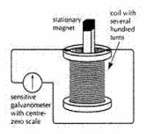
c) no current flow when the magnet is stationary
