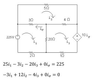
$\begin{aligned} -20i_1 - 4i_2 + 25i_3 + 10i_{\sigma} &= 0 \\ 1i_1 - 1i_2 + 0i_3 + 1i_{\sigma} &= 0 \\ \text{Solving, } i_1 &= 108 \text{ A} \text{ , } i_2 &= 65 \text{ A} \text{ , } i_3 &= 114 \text{ A} \text{ , } i_{\sigma} &= -43 \text{ A} \\ P_{20\Omega} &= (114 - 108)^2 (20) &= 720 \text{ W} \\ P_{10i_{\sigma}} &= 10i_{\sigma}i_3 &= -49.02 \text{ kW} \text{ ,extracted.} \end{aligned}$
