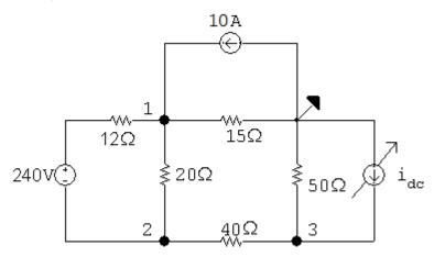
Since the 10 A source is developing 0 W,  $v_1$  must be 0 V.
