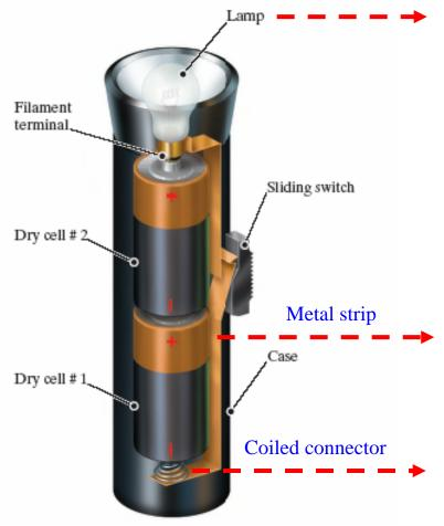
Physics: Filament is heated to a temperature high enough to radiate the visible light. Modeling: a resistor  $R_l$  (only accounts for conversion of electric energy to thermal energy, not light energy).
