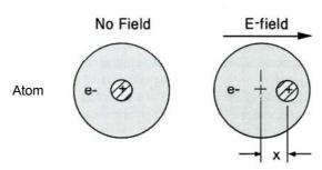
The electric polarization comes from each dipole moment. As in the figure,
