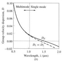
The actual single-mode waveguide dispersion should consider both waveguide dispersion and material dispersion
