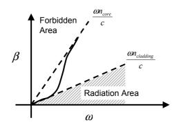
$$\Delta \tau_{g} = \frac{d\beta}{d\omega}\bigg|_{\omega_{1}} - \frac{d\beta}{d\omega}\bigg|_{\omega_{2}}$$
