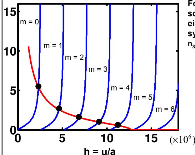
For example, how many solutions to satisfy the eigenvalue equation for a symmetric waveguide ( $n_2 = n_3$ )?
