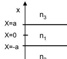
$$\left. \frac{dE_y}{dx} \right|_{x=a^-} = \left. \frac{dE_y}{dx} \right|_{x=a^+} \quad \text{and} \quad \left. \frac{dE_y}{dx} \right|_{x=-a^-} = \left. \frac{dE_y}{dx} \right|_{x=-a^+}$$
