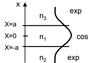
**Boundary Condition 1:**  $E_y$  is continuous at  $x = a$  and  $x = -a$
