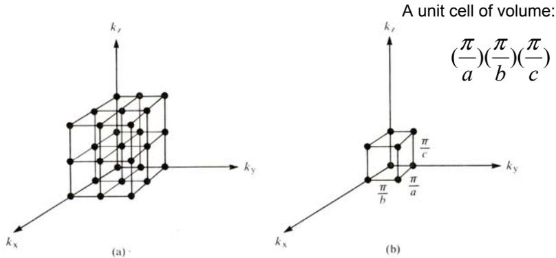
Fig. 4.3 (a)  $k$ -space representation of Schrödinger equation solutions for a particle in a crystal-sized three-dimensional box. (b)  $k$ -space unit cell for solution points.
