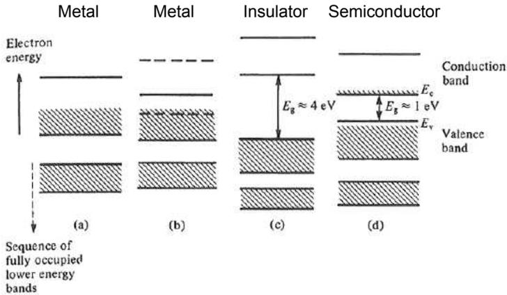
FIG. 2.7 Schematic representation of the energy bands in various materials: (a) a metal with partially filled valence band, e.g. monovalent metals; (b) a metal with two overlapping partially filled bands, e.g. divalent metals; (c) an insulator; and (d) an intrinsic semiconductor. In this, and succeeding diagrams, shading is used to signify occupied electron energy levels.
