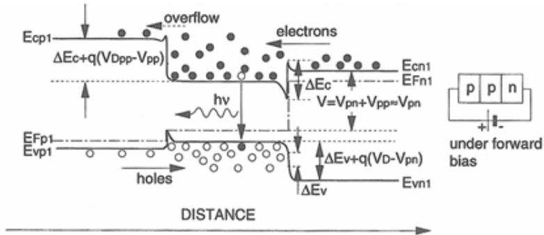
FIGURE 1.47 Energy band diagram of a double heterostructure.
