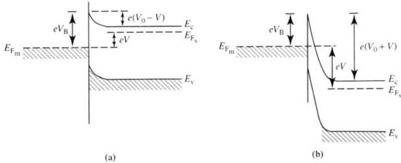
The metal to n-type semiconductor junction shown under (a) forward bias and (b) reverse bias.
