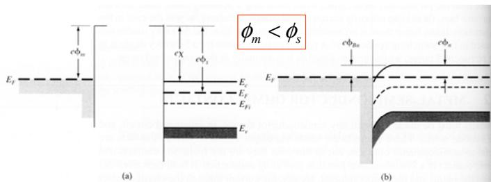
Figure 8.11 Ideal energy-band diagram (a) before contact and (b) after contact for a metal-n-semiconductor junction for  $\phi_m < \phi_s$ .
