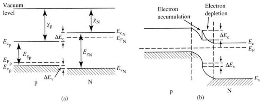
FIG. 2.28 A p-N heterojunction: (a) shows the energy bands of the semiconductors separately; (b) show the energy bands after junction formation. (For a GaAs/Ga<sub>0.3</sub>Al<sub>0.7</sub>As heterojunction,  $E_{sp} = 1.43$  eV,
