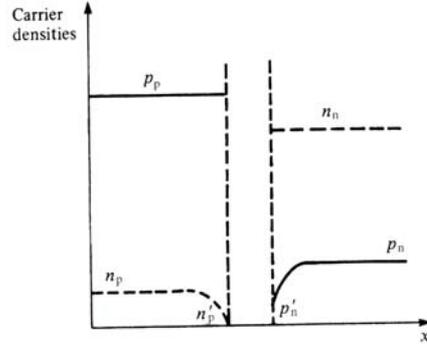
FIG. 2.24 Carrier densities in the bulk regions of a reverse-biased p-n junction. The minority carrier densities close to the depletion layer are shown.
