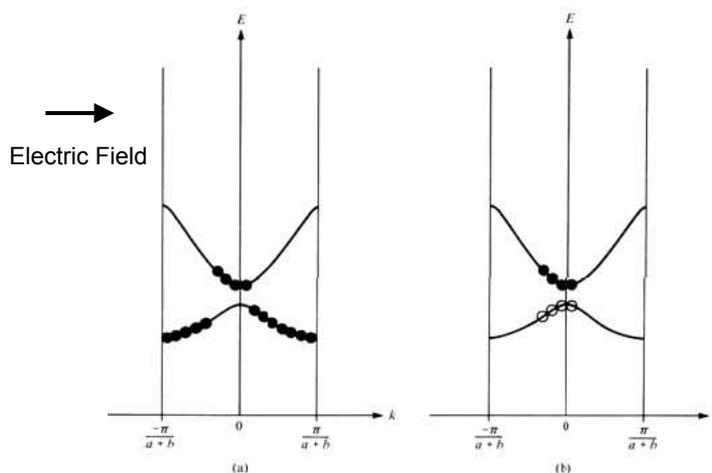
**Fig. 3.11** (a) The skewed filled-state distribution under steady-state conditions subsequent to the application of an external force. (b) Introduction of the hole. Alternative description of the electronic configuration in the lower energy band.
