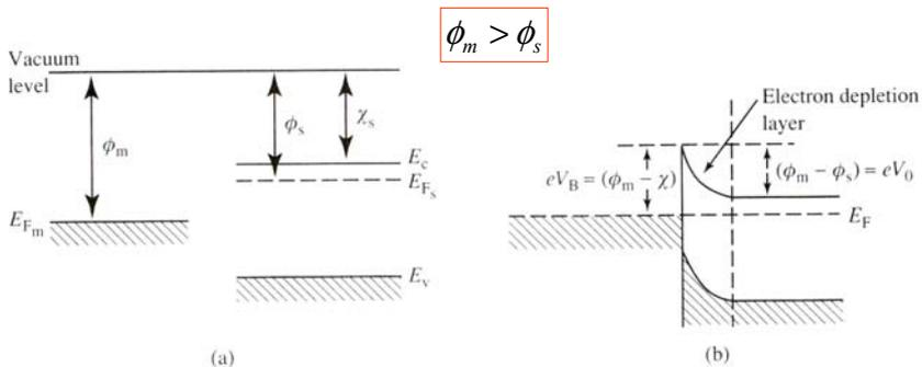
A schottky barrier formed by contacting a metal to an n-type semiconductor with the metal having the larger work function: band diagrams (a) before and (b) after the junction is formed.
