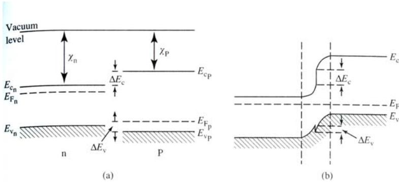
FIG. 2.29 An n-P heterojunction before (a) and after (b) junction formation.
