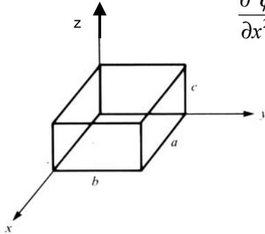
$$\frac{\partial^2 \varphi}{\partial x^2} + \frac{\partial^2 \varphi}{\partial y^2} + \frac{\partial^2 \varphi}{\partial z^2} + k^2 \varphi = 0 \quad (\text{a})$$
