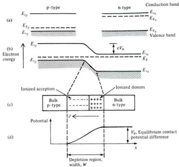
(a). Initially separated p-type and n-type semiconductor;
