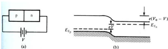
FIG. 2.21 Forward bias voltage  $V$  applied to a p-n junction (a) and the resulting energy band structure (b).
