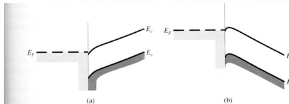
Figure 8.12 Ideal energy-band diagram of a metal-n-semiconductor ohmic contact (a) with a positive voltage applied to the metal and (b) with a positive voltage applied to the semiconductor
