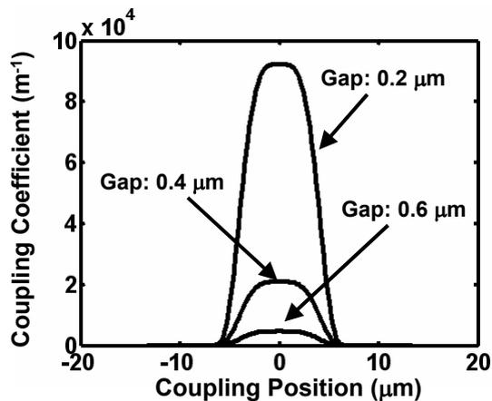
The effective coupling length is only from  $-5\mu\text{m}$  to  $5\mu\text{m}$
