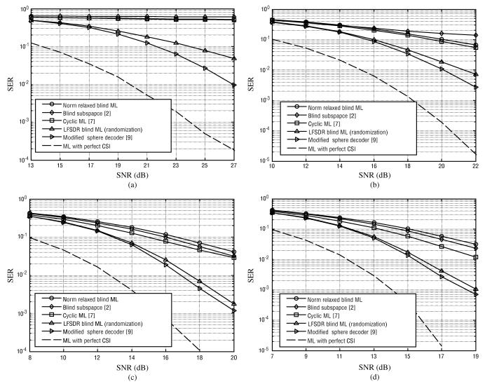
Fig. 5. Performance (SER) comparison results of the proposed LFSDR with some existing suboptimal methods and Cui–Tellambura's modified sphere decoder [9] for various settings. (a)  $N_r = 1$ , P = 2; (b)  $N_r = 2$ , P = 2; (c)  $N_r = 3$ , P = 2; (d)  $N_r = 4$ , P = 2.
