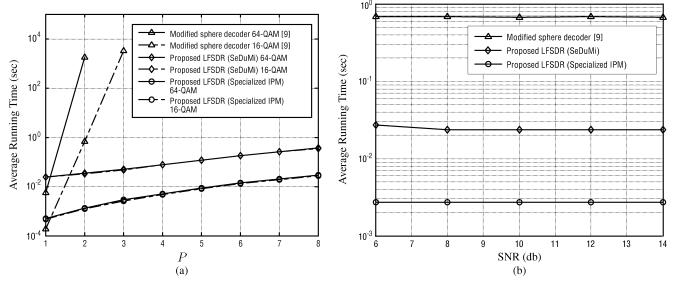
Fig. 4. Complexity comparison results of the proposed LFSDR (solved respectively by SeDuMi [21] and the specialized IPA in Table I) and Cui-Tellambura's modified sphere decoder [9]. (a) SNR = 13 dB,  $N_r = 4$ ; (b) 16-QAM,  $N_r = 4$ , P = 2.
