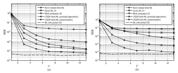
Fig. 2. Performance (SER versus P) comparison results of the proposed LFSDR blind ML detector with some existing methods for the complex  $3 \times 4$  OSTBC. (a) 16-QAM, SNR = 17 dB,  $N_r = 4$ ; (b) 64-QAM, SNR = 23 dB,  $N_r = 4$ .
