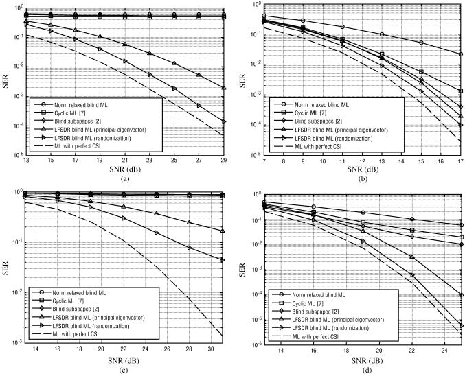
Fig. 1. Performance (SER versus SNR) comparison results of the proposed LFSDR blind ML detector with some existing methods for the complex  $3 \times 4$  OSTBC under various settings. (a) 16-QAM,  $N_r = 1$ , P = 8; (b) 16-QAM,  $N_r = 4$ , P = 8; (c) 64-QAM,  $N_r = 1$ , P = 8; (d) 64-QAM,  $N_r = 4$ , P = 8.
