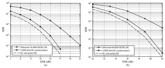
Fig. 3. Performance (SER versus SNR) comparison results of the LFSDR and the differential OSTBC scheme for the complex  $4 \times 4$  OSTBC. (a) 16-QAM,  $N_r = 4, P = 8$ ; (b) 64-QAM,  $N_r = 4, P = 8$ .
