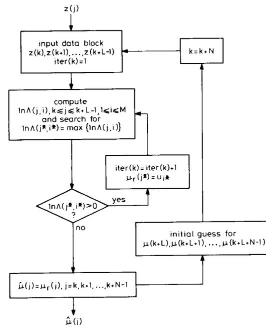
Fig. 1 Signal processing procedure of the proposed recursive SMLR equaliser.
