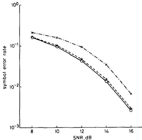
Fig. 2 Simulation results for the infinite one-pole channel with impulse response  $v(j) = 0.9^j$  for  $j > 0$
