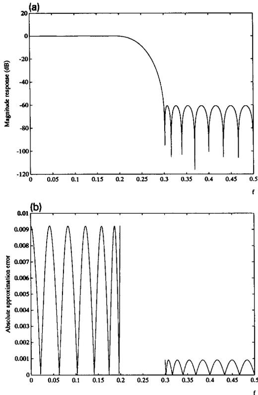
Fig. 2. Example 1. The designed linear phase lowpass filter with  $M=28$  (type II), passband = [0, 0.2] and stopband = [0.3, 0.5]. (a) Magnitude response, (b) absolute approximation error.
