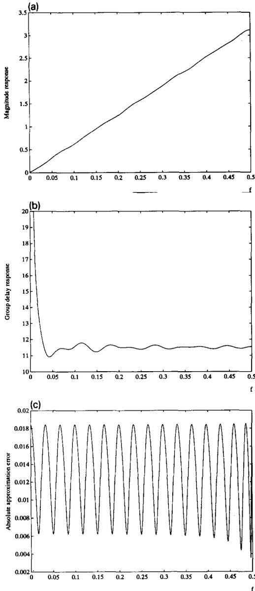
Fig. 4. Example 3. The designed full-band differentiator with  $M=31$  and  $\tau_d=11.5$ . (a) Magnitude response, (b) group delay response, (c) absolute approximation error.
