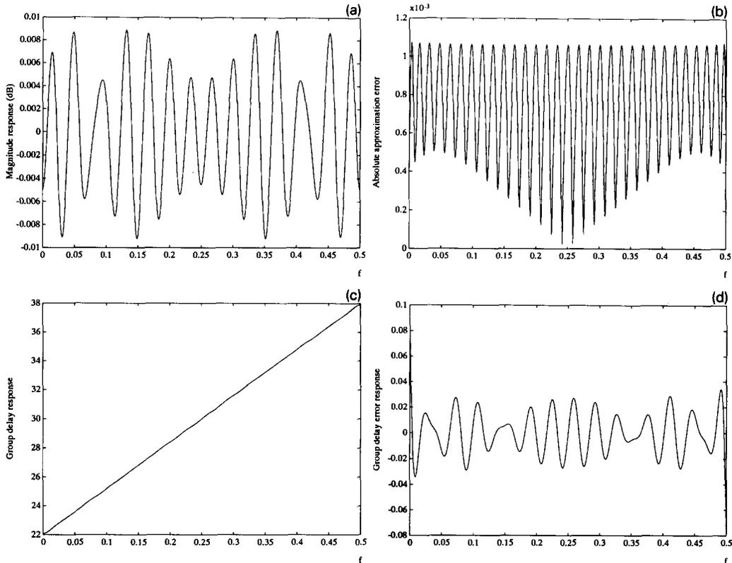
Fig. 5. Example 4. The designed chirp all-pass phase equalizer with  $M=61$ . (a) Magnitude response, (b) absolute approximation error, (c) group delay response, (d) group delay error response.
