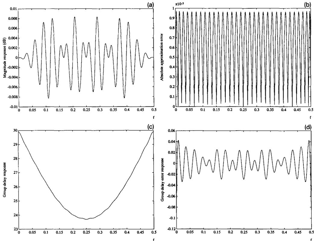
Fig. 6. Example 5. The designed sine-delay all-pass phase equalizer with  $M=61$ . (a) Magnitude response, (b) absolute approximation error, (c) group delay response, (d) group delay error response.
