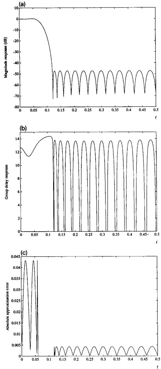
Fig. 3. Example 2. The designed lowpass filter with  $M=31$ ,  $\tau_d=12$ , passband = [0, 0.06] and stopband = [0.12, 0.5]. (a) Magnitude response, (b) group delay response, (c) absolute approximation error.
