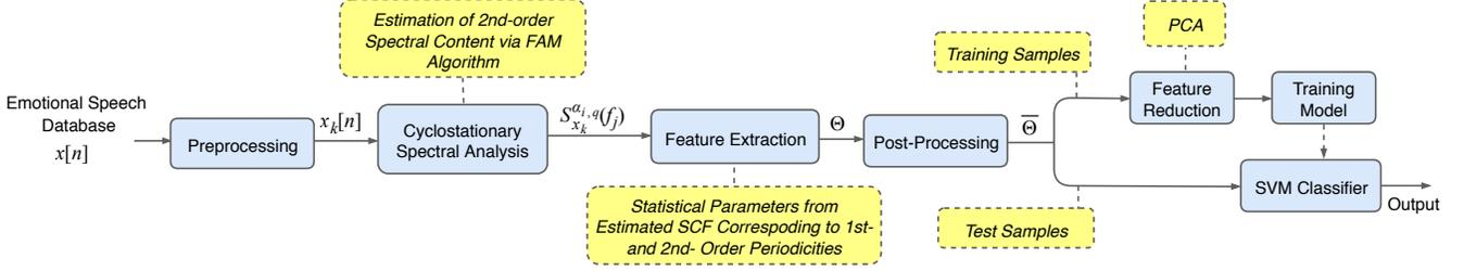
**Fig. 3:** SER system using the proposed CSA based feature extraction scheme
