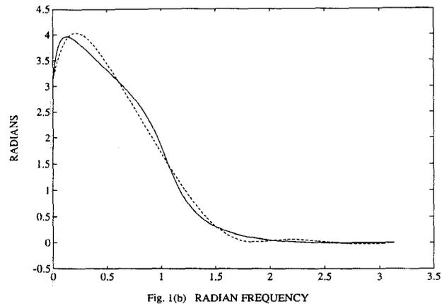
**Fig. 1.** Simulation results associated with Example 1 for SNR = 10 and  $N = 1024$ . (a) Thirty system phase estimates  $\hat{\theta}(\omega)$  with the unknown linear phase factor artificially removed for each estimate; (b) the average (dashed line) of the thirty estimates shown in Part (a) and the true system phase response (solid line).
