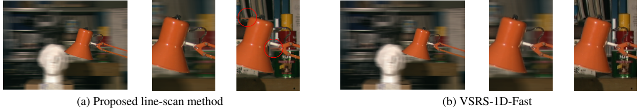
Fig. 5. 1-D aperture refocusing for the central 5 \times 1 light field of Tsukuba with D = 9.75 and n = 8 (Left: refocused image; Middle: cropped image; Right: cropped novel view at v = -11/8 ). Both refocusing images look good and have no obvious artifacts. The proposed line-scan would generate novel views with streak artifacts. Some worst cases are shown here at v = -11/8 , which get blurred in the refocused image.
