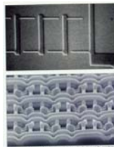
Figure 8.38 Electromagnetically-related failure modes (Courtesy of N. Cheung and A. Tai, U.C. Berkeley)
