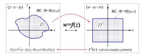
The strategy works because harmonic functions remain harmonic under conformal mapping. Proof: f(z) and  $F^*(w)$  are analytic (s.t. Re $\{F^*(w)\}$  is harmonic). By the chain rule, F(z) is also analytic:  $F'(z) = \frac{dF^*}{dw} \cdot f'(z) \Big|_{w=f(z)}$  exists.  $\Rightarrow \Phi(x,y) = \text{Re}\{F(z)\}$  is harmonic.
