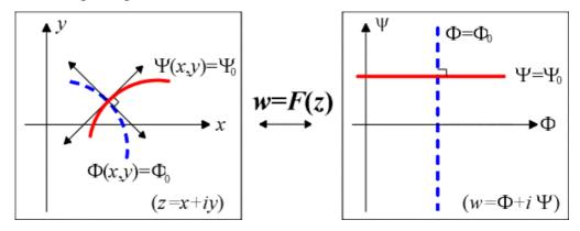
Since gradient defines the steepest ascent/descent direction, which is always perpendicular with the equipotential lines (zero-variation direction),  $\Rightarrow$  E-field  $\vec{E} = -\nabla \Phi$  is perpendicular with  $\Phi(x,y)$ =constant,  $\Rightarrow \Psi(x,y)$ = $\Psi_0$  stands for a E-field (force) line.
