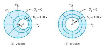
Direct solution in the z-plane is difficult. By using linear fractional transformation:  $w = f(z) = \frac{z - 1/2}{(z/2) - 1}$  (EK 17.2–17.4), domain D is mapped onto  $D^*$  in the w-plane, consisting of two concentric circles:  $C_1^*$ : |w| = 1,  $C_2^*$ :  $|w| = \frac{1}{2}$ ; with BCs:  $U_1 = 0$ ,  $U_2 = 110$ .
