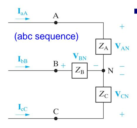
The instantaneous powers of  $Z_A$ ,  $Z_C$  are:  $p_B(t) = v_{BN}(t)i_{bB}(t)$  $=V_m I_m \cos(\omega t - 120^\circ)$  $\cos(\omega t - \theta_{\phi} - 120^{\circ}),$  $p_{C}(t) = V_{m}I_{m}\cos(\omega t + 120^{\circ})$  $\cos(\omega t - \theta_{\phi} + 120^{\circ}).$
