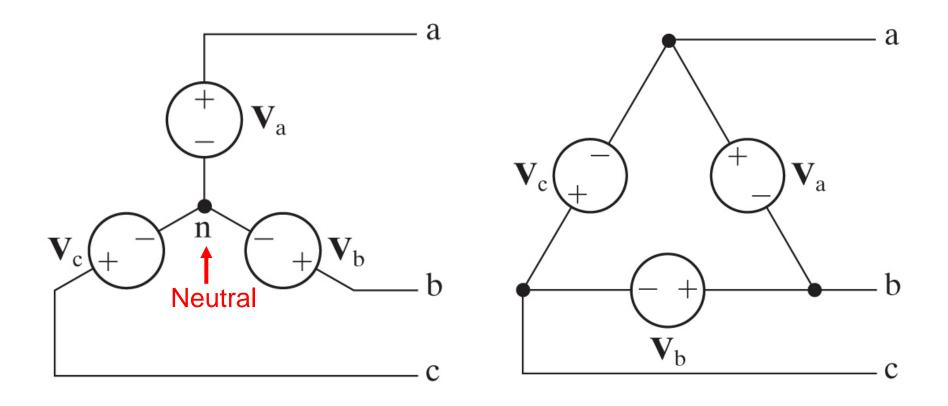
Real Y- and  $\Delta$ -connected voltage sources
