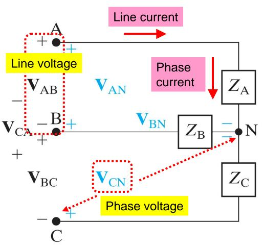
For Y-connected load, line current equals phase current.
