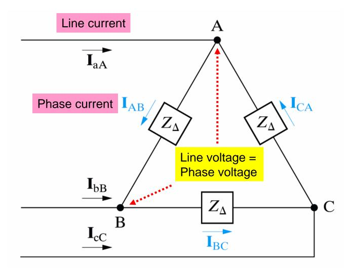
$\Delta$ -Y transformation for balanced 3-phase load
