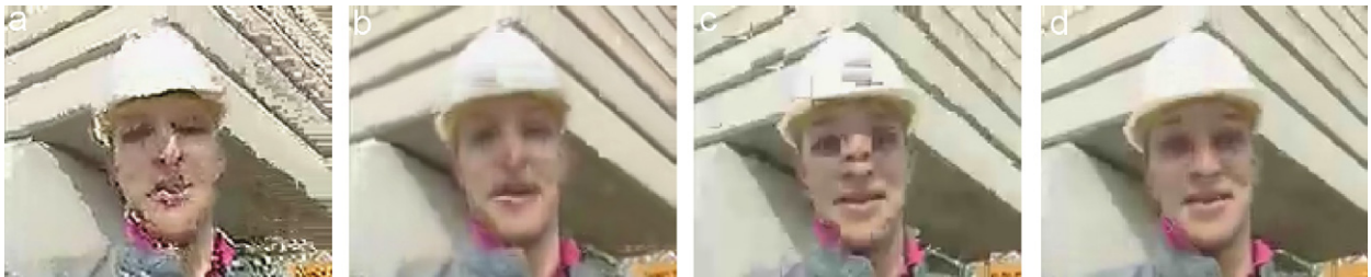
Fig. 14. Subjective performance comparison of different methods for frame #80 of Foreman (PLR = 5%, error pattern #2, QP = 36): (a) Inter-MCP (14.33 dB), (b) 2HMCP (19.91 dB), (c) Inter-MCP with 20% IR rate (26.06 dB), and (d) the proposed 2HMCP with 10% IR rate (30.18 dB).
