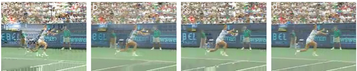
Fig. 15. Subjective performance comparison of different methods for frame #185 of Stefan (PLR = 5%, error pattern #2, QP = 36): (a) Inter-MCP (17.00 dB), (b) 2HMCP (23.42 dB), (c) Inter-MCP with 20% IR rate (23.47 dB), and (d) the proposed 2HMCP with 10% IR rate (26.86 dB).
