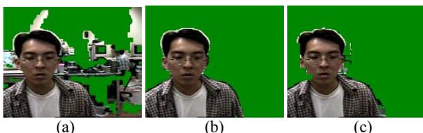
Fig. 6. (a) segmentation without template matching, (b) previous segmented result used as the template, (c) refined segmentation result after template matching.
