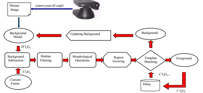
Fig. 3. Procedure of active video object tracking.
