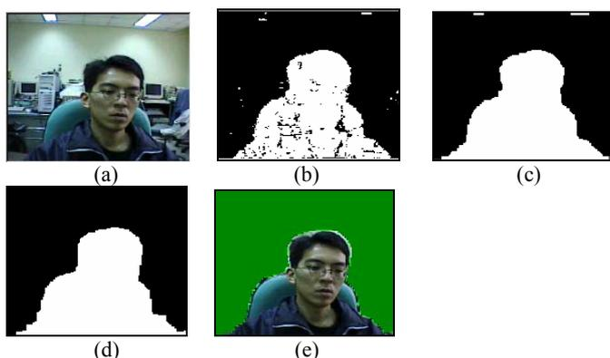
Fig. 4. Simulation result of the proposed object discrimination: (a) the incoming image; (b) alpha plane obtained by background subtraction; (c) alpha plane after post-filtering; (d) alpha plane after region growing; (e) final segmentation result.
