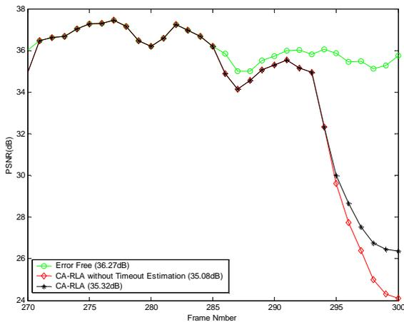
Fig. 6. Frame-by-frame PSNR performance comparisons of the CA-RLA with and without timeout estimation at  $n_{ms} = 8$  and  $\beta = 9$ .
