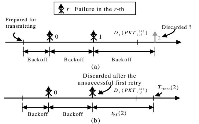
Fig. 4. Illustrations of two packet scheduling scheme: (a) the traditional method without backoff time estimation and (b) the proposed scheduling method based on backoff time estimation.
