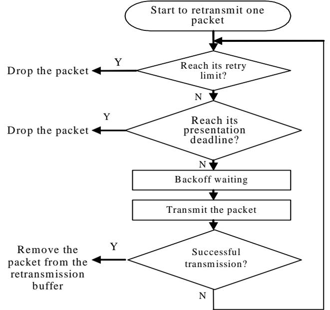
Fig. 3. Flowchart of retransmission-based packet scheduling in CA-RLA.
