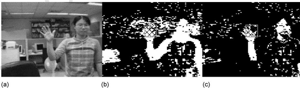
Fig. 3. (a) The origin frame, (b) extracted skin regions satisfying R > G > B , and (c) compare the colors of the extracted skin regions with the sample skin color.
