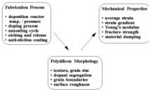
Fig. 1. Microstructural polysilicon mechanical property dependency on film morphology and fabrication process parameters.
