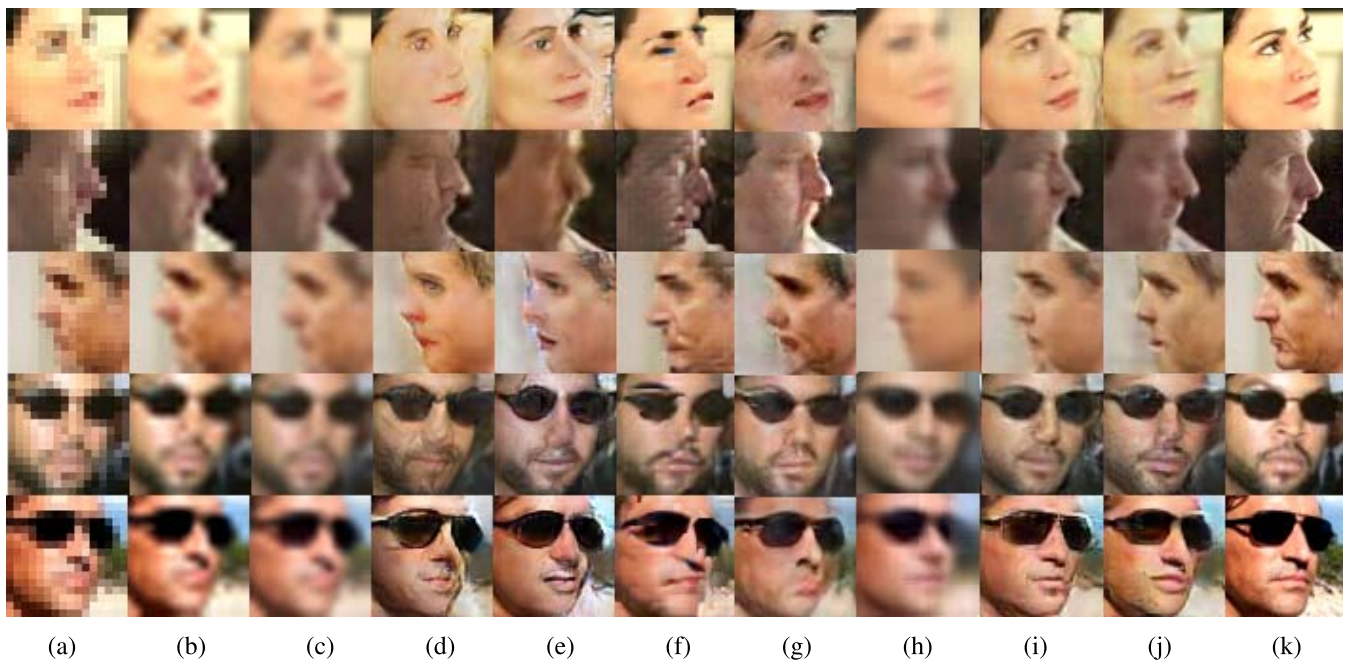
Fig. 8. Subjective visual quality comparison for five faces with unknown identities selected from LFW [28] and CelebA [29]: (a) the LR face images ( 16 \times 16 ), (b)–(j) the reconstructed 64 \times 64 HR faces using (b) bicubic interpolation, (c) DFCG [11], (d) DCGAN [22], (e) UR-DGN [9], (f) PRSR [25], (g) SR-GAN [15], (h) Wavelet-SRNet [17], (i) SiGAN (DenseNet), (j) SiGAN (ResNet), and (k) the ground-truths ( 64 \times 64 ).
