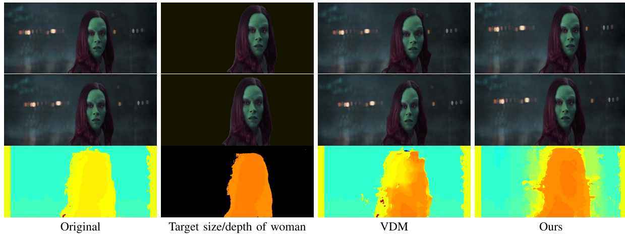
Fig. 11. Comparison of our method and VDM [6] on Woman in movie Guardians of the Galaxy , where the size and depth of the woman is increased. From top to bottom: the left-view image, right-view image, and the disparity map. The 2nd column shows the selected object where its size is adjusted to a target size in the 1st and 2nd row, and its ground-truth depth is showed in the 3rd row.
